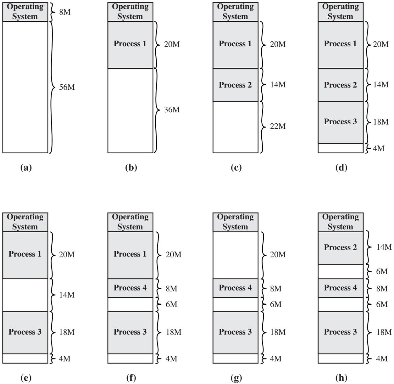
**Figure 7.4 The Effect of Dynamic Partitioning**
