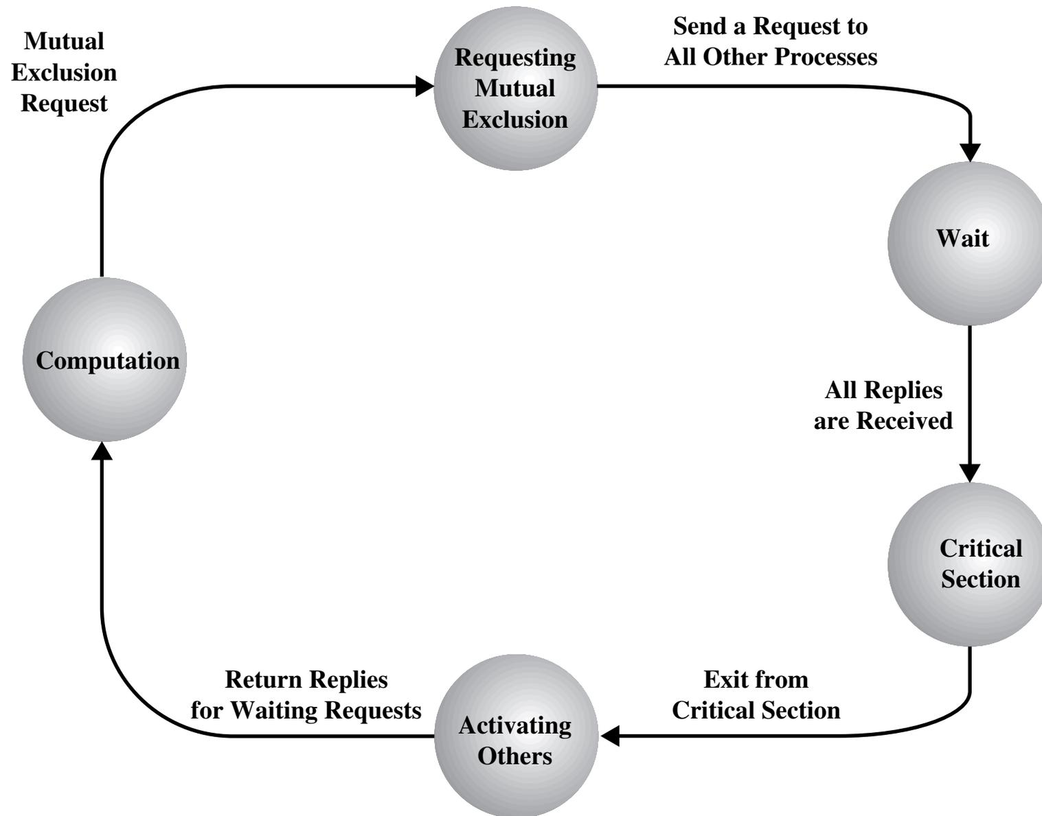
**Figure 14.10 State Diagram for Algorithm in [RICA81]**
