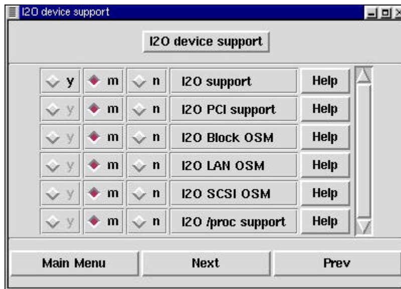
Figure 2. Kernel compilation options for I 2 O modules
