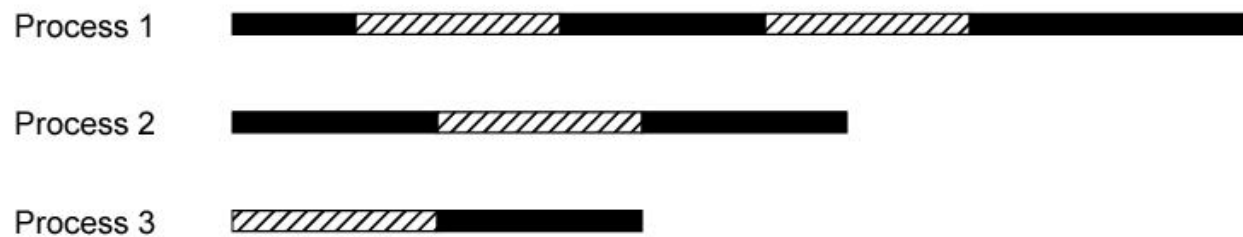
(b) Interleaving and overlapping (multiprocessing; multiple processors)
