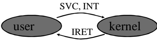
The diagram shows two ovals labeled 'user' and 'kernel' connected by two curved arrows. The top arrow points from 'user' to 'kernel' and is labeled 'SVC, INT'. The bottom arrow points from 'kernel' to 'user' and is labeled 'IRET'.
