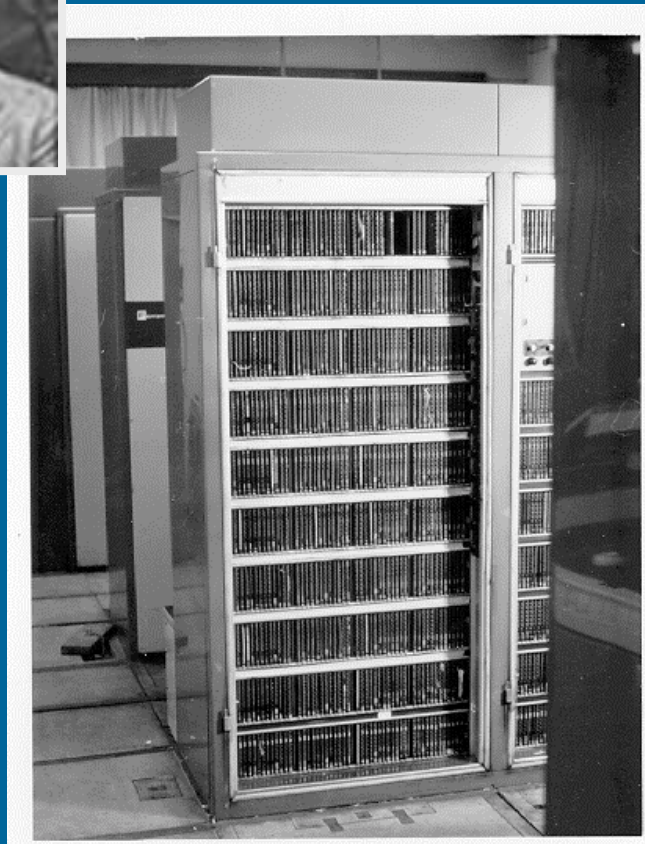
Atlas accumulator cabinet
