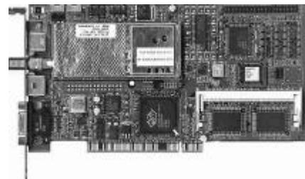
(PCI card - connectors also on other side, some pins not used by this card)
