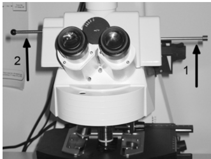
Figure 3. Rods controlling the oculars/camera light path.
