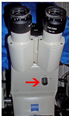
Figure 5. Ocular light path adjustment.
