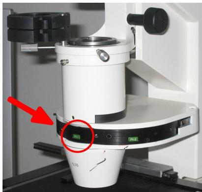
Figure 7. The position of the condenser.
