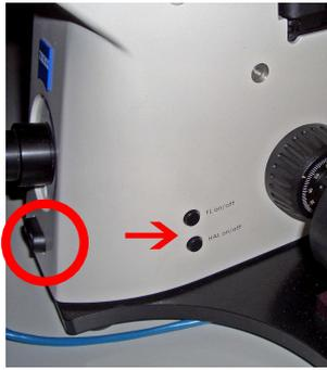
Figure 6. Red arrow: on/off button for transmitted light.
