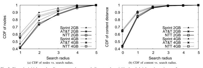
Fig. 3: Given the initial search radius preset to the network diameter, the neighborhood shrinks to its optimum after convergence. In practice, the optimal neighborhood is small and most content is retrieved from the neighbors within 2 hops.
