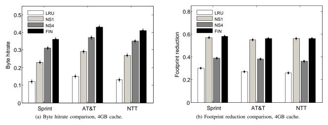
Fig. 6: Performance evaluation of four caching strategies on three realistic ISP networks.
