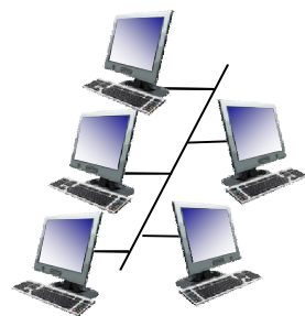
shared wire (e.g., cabled Ethernet)
