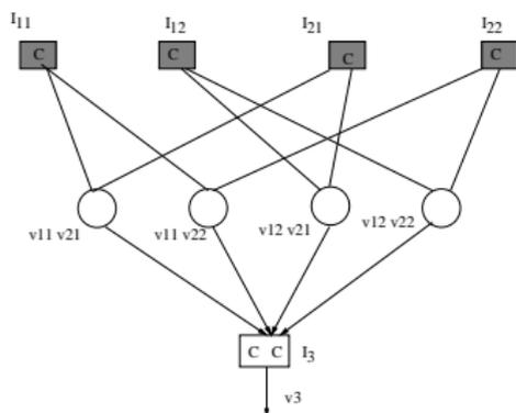
$$v_3 I_3 = v_{11} v_{21} I_{11} I_{21} + v_{11} v_{22} I_{11} I_{22} + v_{12} v_{21} I_{12} I_{21} + v_{12} v_{22} I_{12} I_{22}$$
